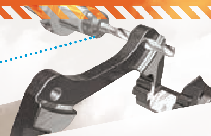
4 Special Side Cutter [ Housing Head ] : Facing-Roughing, finishing
